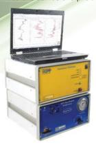
This injection pressure log is an excellent indicator of formation permeability. In addition to measurement of injection pressure, the HPT can also be used to measure hydrostatic pressure under the zero flow condition. This allows the development of a hydrostatic pressure graph for the log and prediction of the position of the water table.
