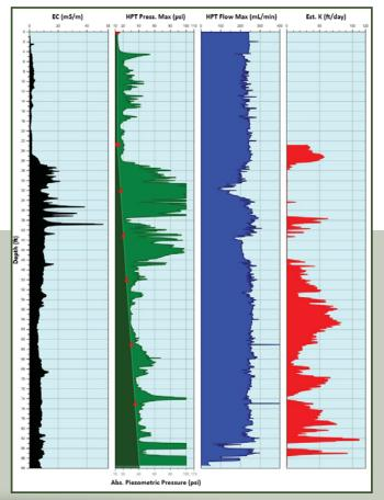
Measurement of the injection pressure in the HPT system is made using a downhole pressure transducer. Use of a transducer in the downhole position allows measurement of the injection pressure at the HPT screen only and excludes frictional losses through the flow tube of the HPT trunkline. The downhole transducer position is also necessary for making hydrostatic pressure measurements at the probe.
